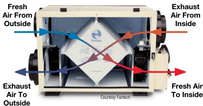
cook stove hoods? This is definitely not recommended or permitted. Both sources have contaminants in the airstream that will foul the heat exchanger and decrease its efficiency. Furthermore, there are fire risks associated with cooktops and their combustion products. The heat recovery potential from an intermittent exhaust source is negligible, since residential appliances do not continuously run.
